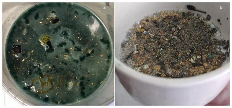
Figure 6: Leaching of solder: **a** detached gold sputtering on the surface of PLS, **b** gold, silver sputtering and electronic components
