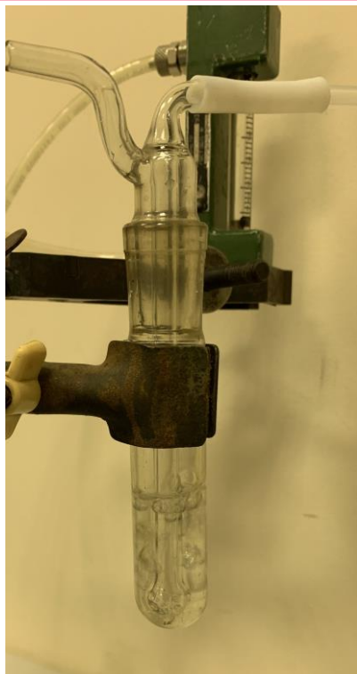
Figure 7 - The process of gas dissolving by bubbler using
