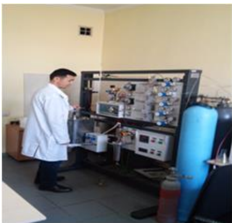
Flow type PKU-2VD catalytic installation
