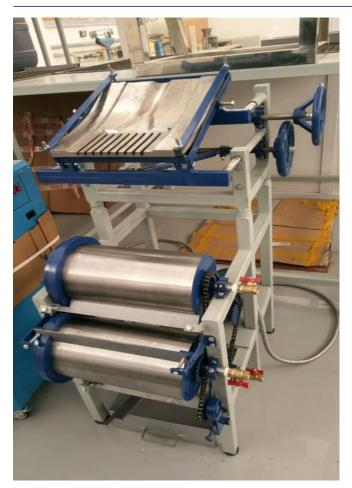
Appearance of laboratory granulator for dry granulation of slag melts.
