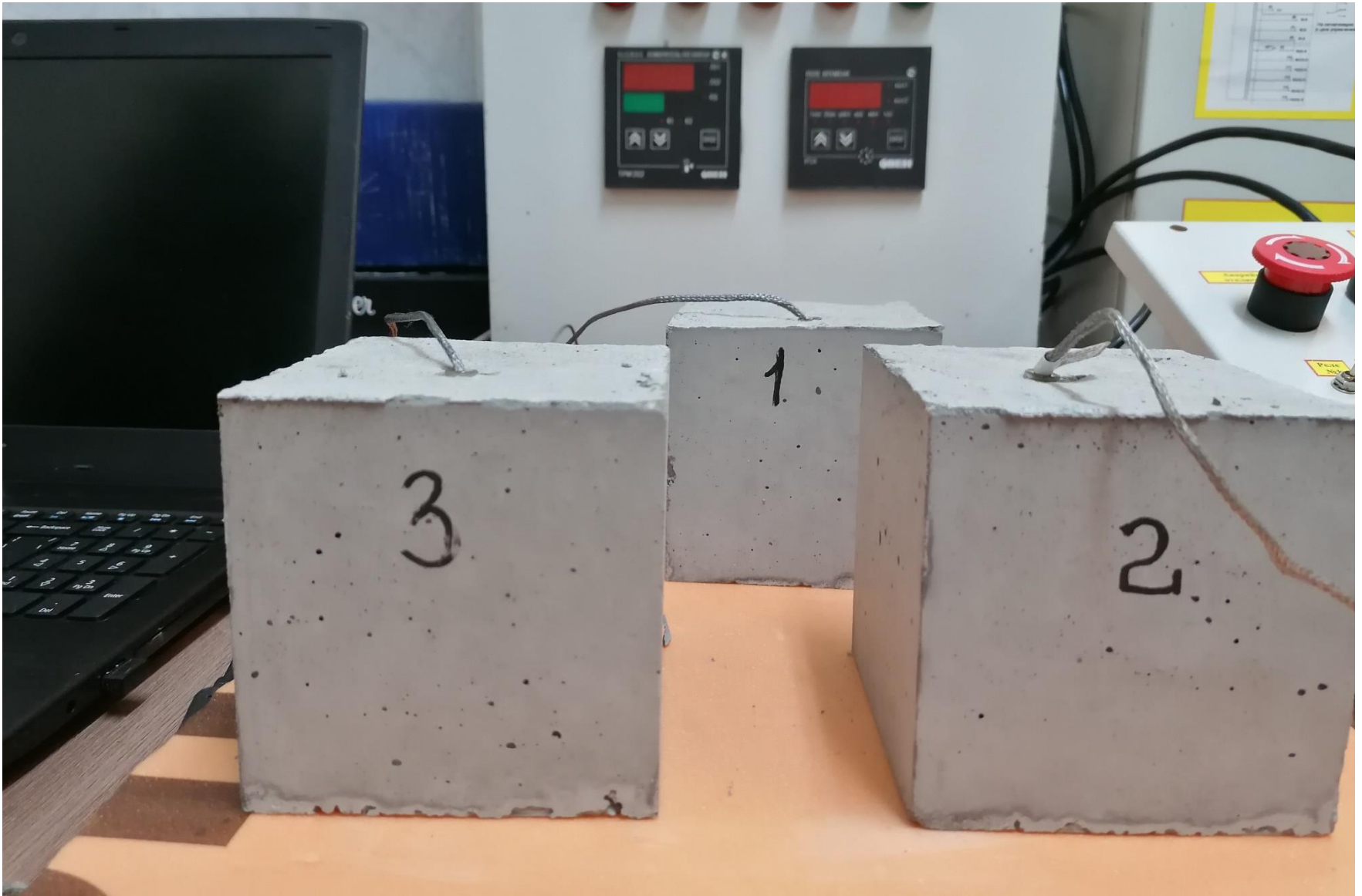
Samples after demolding. Natural cooling phase.
